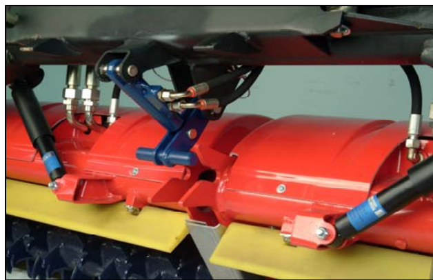
Photo 2.23 Flex tiller lockout device
