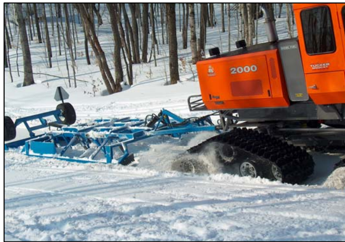
Photo 4.13 Beware of trenches dug by spinning tracks
