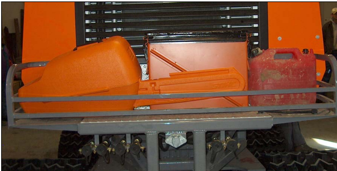
Photo 2.30 Typical cargo deck used to carry tools, spare signs, and spare fuel
