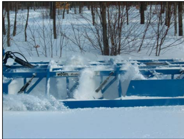
Photo 4.5 Keep processed snow inside the drag!
