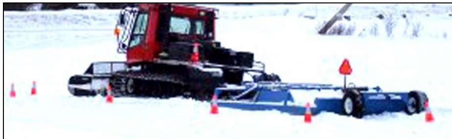
Photo 3.3 Place cones or other warning devices around and in advance of a groomer that has broken down on the trail and must remain there for an extended period.
