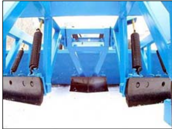
Photo 2.5 Spring tripping blades
